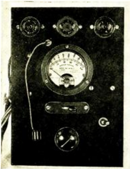
Fig. A Panel view of the versatile, direct-reading, mutual conductance meter designed by Mr. Potts
