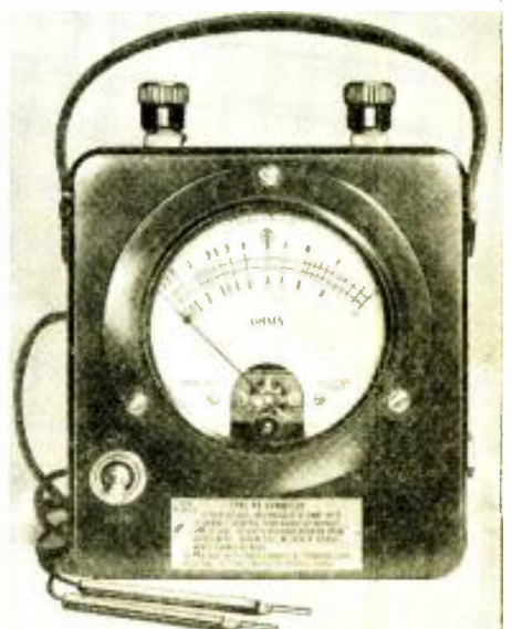
Fig. 11. The Westinghouse ohmmeter. The toggle switch selects the proper range.
